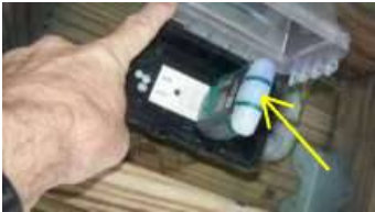
Photo 46-1 Middle light on electric detector should be green
